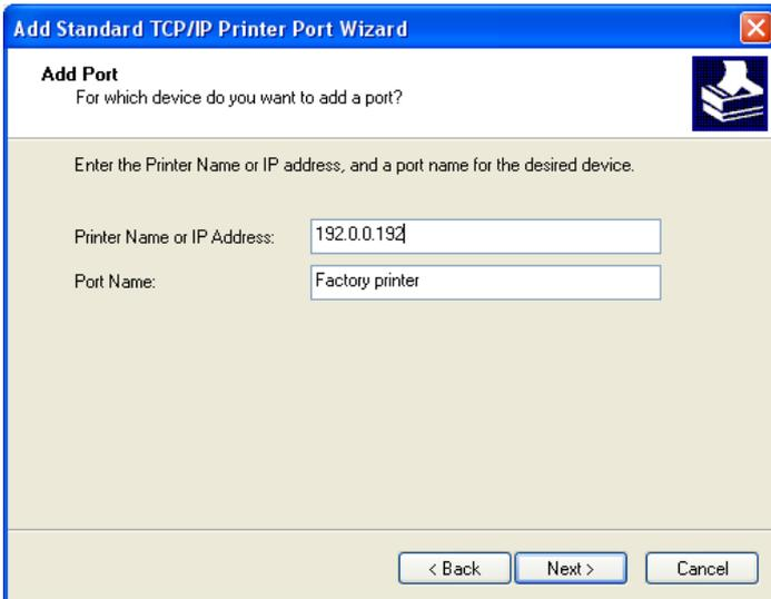
Input the Units IP address or Printer name that you have previously selected. Any descriptive printer name can be used. Click **Next**
