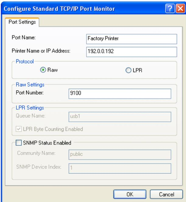
The following Port numbers can be used to print from each physical output port or printer set up on the unit.
