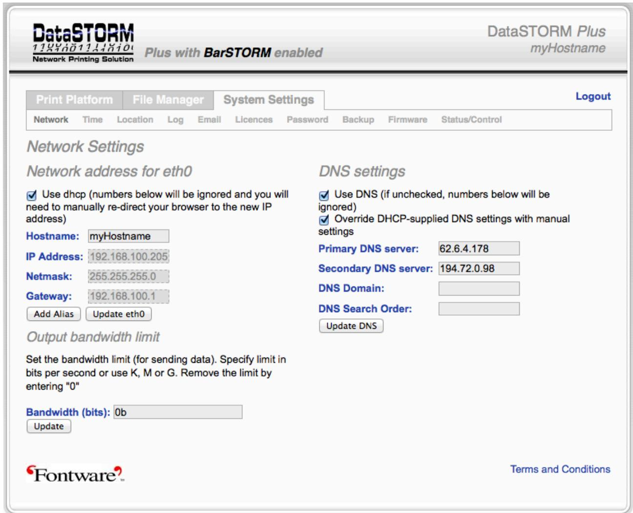
This screen will allow you to change the units Hostname, IP address, Netmask and Gateway information where necessary.
